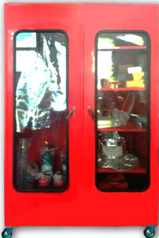
Type : Box Fire Cabinet Size : 180 X 130 X 60 Cm Plate : 1,2 mm Mild Steel Production Process : Dust Remover, Phosphating & Zinc Chromate Primes
