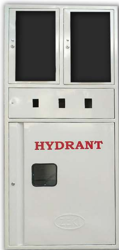
Type : B (customize) Size : 175 X 75 X 20 Cm Plate : 1 mm Mild Steel Production Process : Dust Remover, Phosphating & Zinc Chromate Primes
